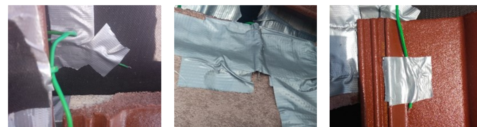
Figure 2-4. Thermocouples on the AWL and on lower surface and upper surface of the roofing [7]
